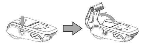
2) Load the roll paper in the orientation shown in the figure below.
