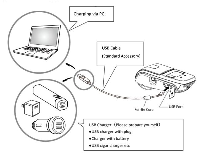
When battery pack runs out of power, the battery icon will flash. It powers off automatically when continues printing. If you want to go on, please charge it.
