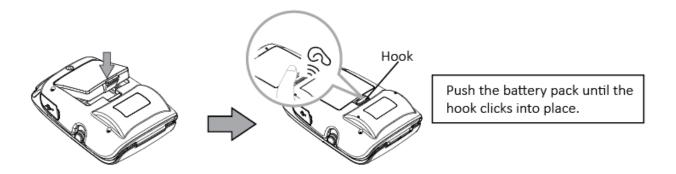
3. To remove the battery back, pull back the hook, and use the opposite procedure from the one you used to insert the battery pack.
