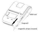
Make sure the magnetic stripe is towards to the magnetic head. Hold the card in the center as illustrated below and swipe it straight at a steady speed in the direction of arrows.
