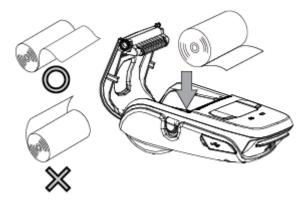
3) Pull the end of the roll straight toward you. Then press down on both sides of the printer cover to close it firmly. When you close the printer cover, make sure that it is closed on both sides.
