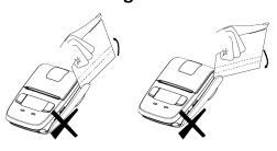
If you insert a card tilted upward/downward into the MSR slot,the card does not move horizontally and a read error occurs.
