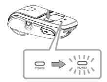
2.To put the printer into Memory Switch Setting mode, press and hold both the MODE & FEED buttons for 5 seconds. After printer displays "Enter Menu Mode", you can configure the settings. Release the buttons after you surely confirm the screen display "Enter Menu Mode", to get a printer into the setting mode.
